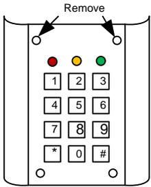
2) Remove the top two security screws as shown. Do NOT remove the bottom screws.
