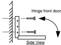
3) Use appropriate wall fixings. 8-10mm anchors, 75mm deep with M5 screw are recommended as a minimum.
